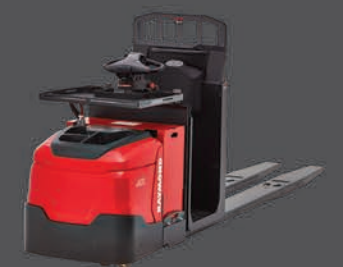
8720 2ND LEVEL ORDERPICKER WITH ELEVATED OPERATOR PLATFORM
